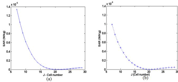
Figure 1. Variation of SAR<sub>1g</sub> in the brain at 100 MHz using, (a) Cubical box model (b) Spherical model.
