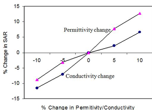
Figure 7. SAR sensitivity for perturbations of Permittivity and Conductivity
