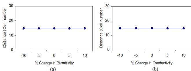
Figure 8. Locations of maximum SAR with respect to the percentage change in: (a) Permittivity with  $\sigma$  remain unchanged (b) Conductivity with  $\epsilon_r$  remain unchanged.
