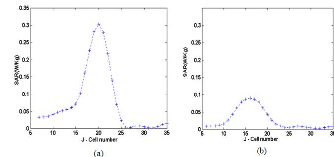
Figure 2. Variation of SAR<sub>1g</sub> in the eye at 2500 MHz for, (a) Spherical model (b) Cubical box model.
