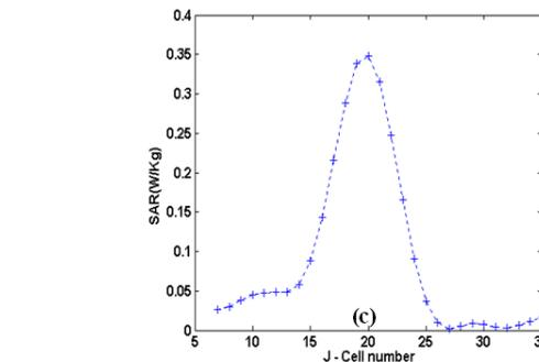
Figure 6. Variation of SAR<sub>1g</sub> in the eye for (a) normal size (b) 5% increased (c) 5% decreased
