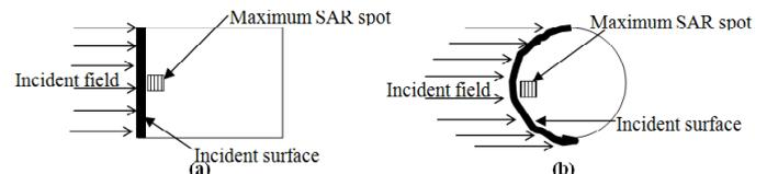
Figure 3. Maximum SAR spot and the incident surface of the brain with (a) cubical box model (b) spherical model.
